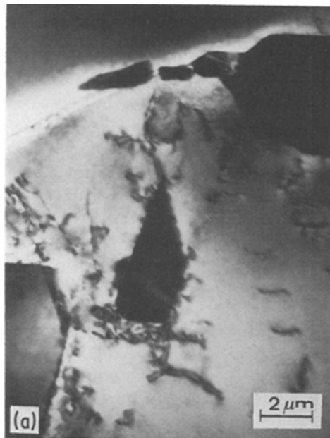
Figure 2 (a) Transmission electron micrograph of carbide precipitation in AISI type 316 sensitized and carburized steel. (b) and (c) SADP taken from M_{23}C_6/\gamma interface and schematic key diagram. ●, M_{23}C_6 ; □, \gamma .
